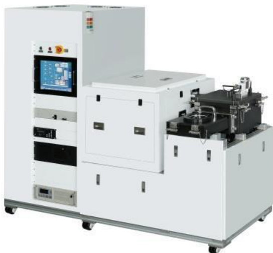
Fig. 1. Plasma ALD tool from CN1.
